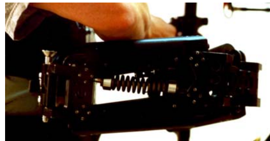
Figure 20 IIA Arm Base Spring
