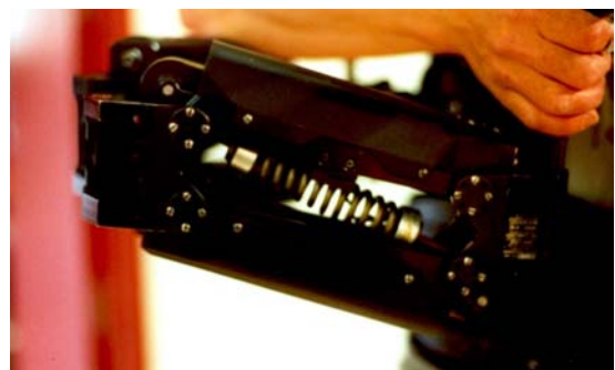
Figure 21 IIA Arm Top Spring
